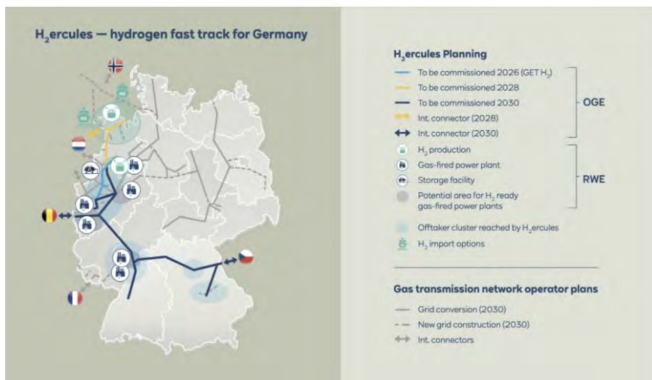
Figuur 57: H 2 ercules. The hydrogen fast track. 105
